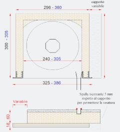
For internal flush in the wall window fixtures with external mortar finish
