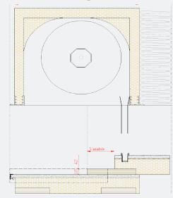
For center wall window fixtures with external exposed brick finish
